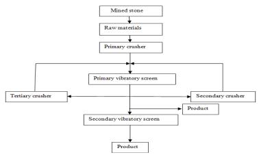
Fig. 1. Stone crushing process flow
